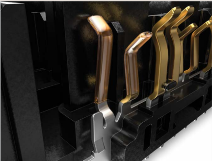
High-cycle "super lube" for extreme mating cycles
