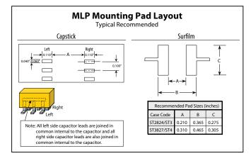
Depending upon pad geometry, the recommended solder paste thickness is .006" (6 mils) to .010" (10 mils). For optimum performance, 8 mils to 10 mils should be used. In the case where small pitch components do not allow extra paste thickness, use of a "step screen" should be considered.
