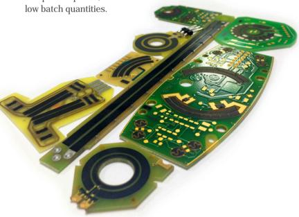
Once screened and cured, these resistive tracks can be individually laser trimmed to obtain very accurate tolerances in high volume.
