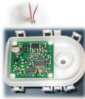
Control for urea injection
