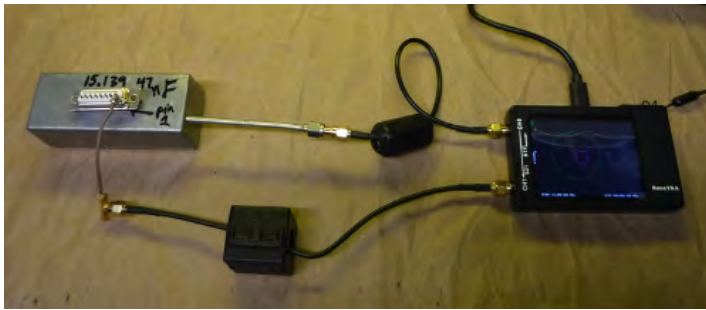
Figure A : NanoVNA , Port0 to interior of pseudo or artificial DUT shielded enclosure DB15 connector pin 1, Port 1 flexible coax to removable DB15 connector. USB cable to Personal Computer running NanoSaver control Application software.
