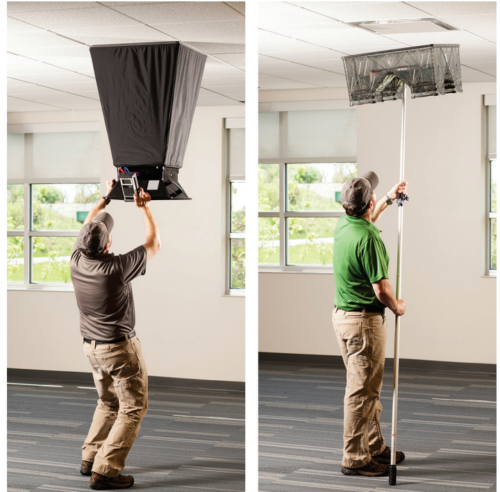
Figure 1 – Traditional air flow hood (left picture) versus Dwyer SMART Air Hood® balancing instrument (right picture)
