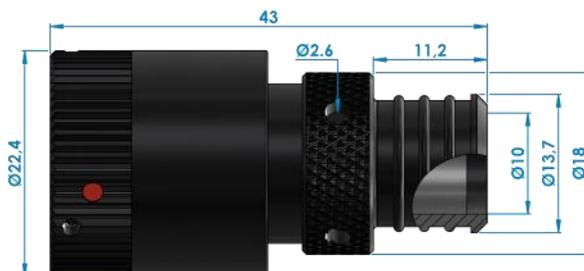
Backshell for cable assembling with metallic collar and heat-shrink boot (not included)
