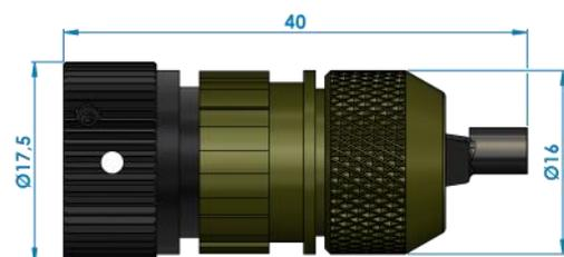
◆ Type 'P' with straight backshell and sleeve
