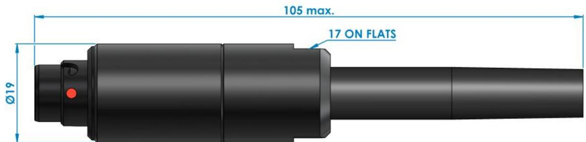
The backshell of PAM 07 FNB1 can be also mounted on extension, part number : PAM 07 PNB1
