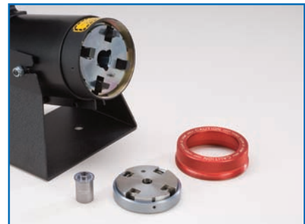
3. Pull out the Locator by hand.
