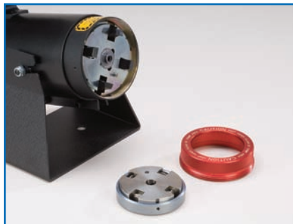
2. Pull off Indenter Die Assembly by hand.
