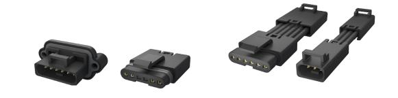
All Plastic with IP67 Sealing Gaskets 3 & 6 Position Housings, Select Loading Crimp or Poke-In Wire Terminations Solid or Stranded Wire, Up to 7A per Pin
