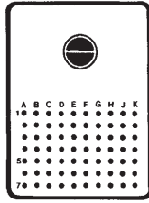
Insert 71W1A (70) Size 22 Contacts (1) Size 1 Coax Contact
