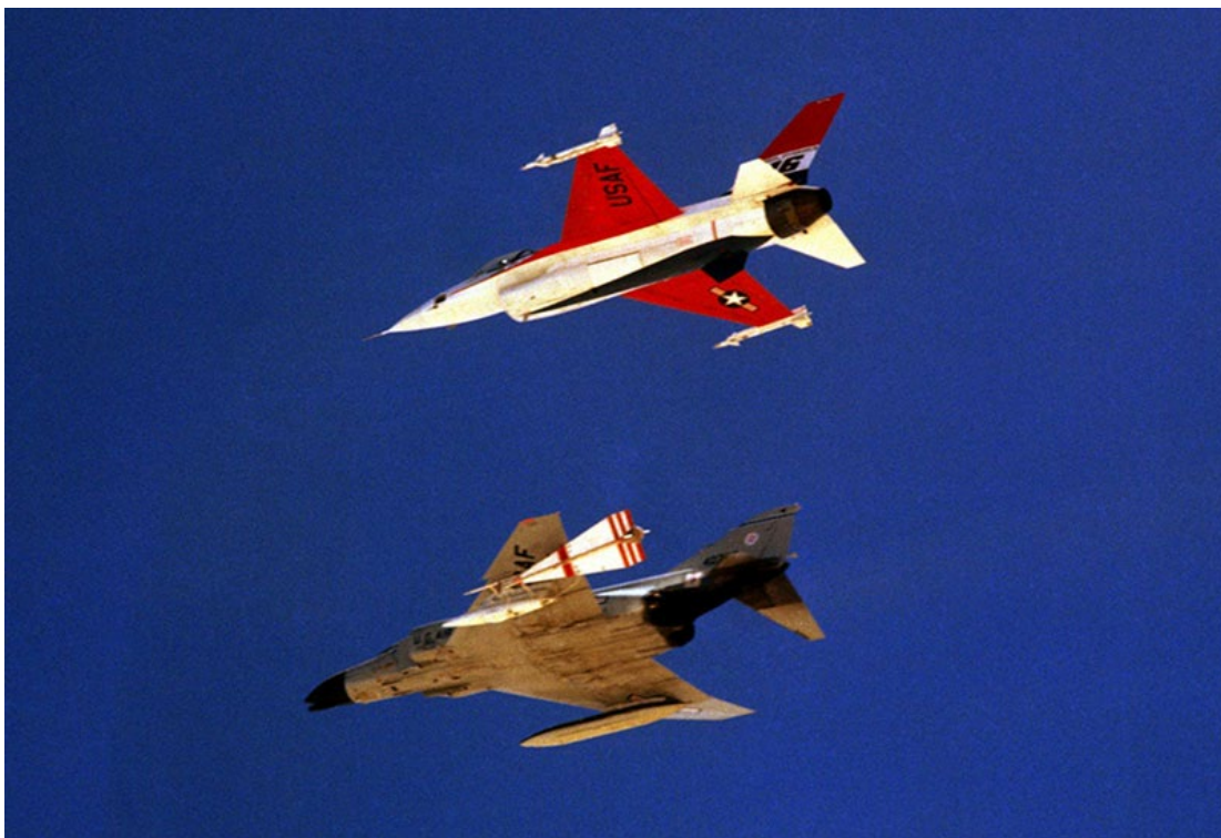
A General Dynamics YF-16 prototype (top) flies in formation with a McDonnell Douglas F-4C Phantom II in 1976. Notice the size difference—a key distinction between third- and fourth-generation aircraft, with the former placing greater emphasis on what we now refer to as SWaP-C principles.
