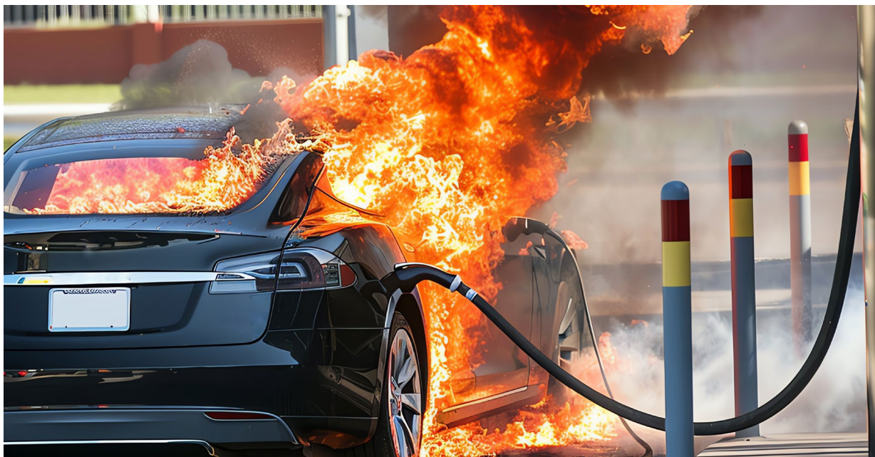
Figure 1: Most electric vehicles use lithium ion battery packs, which carry a risk known as thermal runaway that can cause them to ignite or explode. Image used courtesy of Adobe Stock
